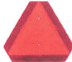
**NOTE** – Slow Moving Vehicle signs significantly increase rearward equipment visibility and also help to ensure that equipment remains operational during daylight hours in the event that a beacon or other HVL fails. Slow moving vehicles working for/with the City of Winnipeg's Public Works Department are to be equipped with both HVL and slow moving vehicle signs.
